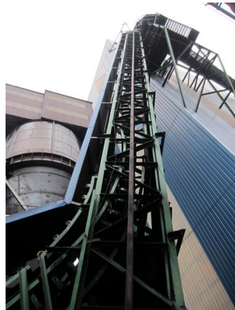
The DSI Sandwich Belt conveyor replaced a problematic pocket belt system eliminating carry back and clean up problems by scraping belts clean.
